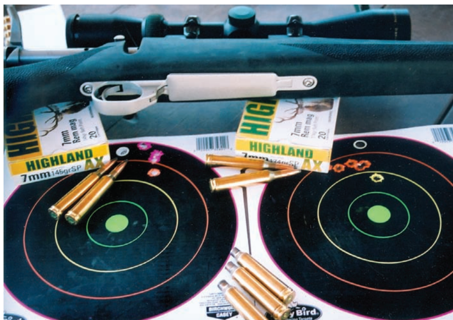
ABOVE: Five-shot groups with 174gr Highland AX ammo (left) printed a bit higher at 100 metres than the 145gr stuff, but accuracy was very good for an untuned factory rifle with commercial ammunition.
