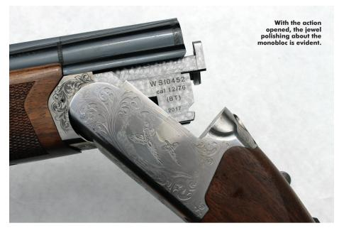
The fore-end was of a Schnabel-style with a typical tulip head to the front. This was generously covered with chequering at around 20 lines per inch. It was obviously completed by laser-guided machinery for there was a single border with no overruns. Inletting of the fore-end catch was admirable with no gaps and the catch was adjusted perfectly to hold the wood firmly to the barrel set.
