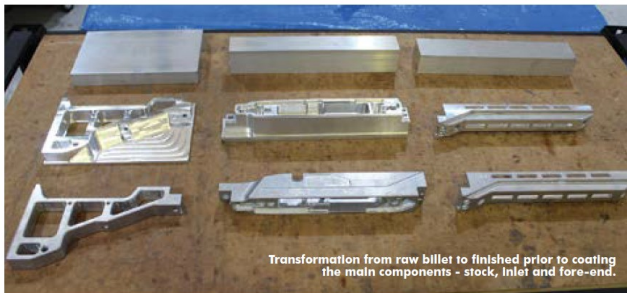
TSP X chassis components at various stages of completion.
