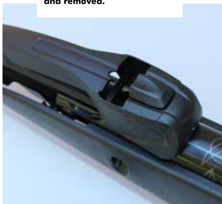
10-shot magazine positioned in the barrel magazine well and removed.
